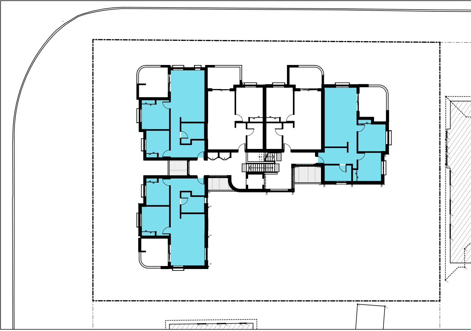
11 - FIRST FLOOR - NATURAL VENTILATION 1:300
